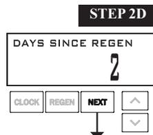
**STEP 2D** – Days, since last regeneration: This display shows the days since the last regeneration occurred. Press NEXT to go to Step 3D. Press REGEN to exit Diagnostics.
